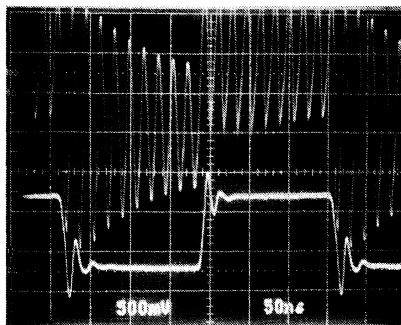
Driving a pure capacitive load. Top trace is without a snubber. Bottom trace is with a snubber circuit.
